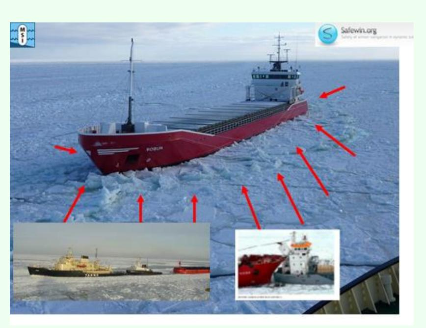
• A ship stuck in compressive ice (red arrows) and needs the icebreaker assistance to proceed further
