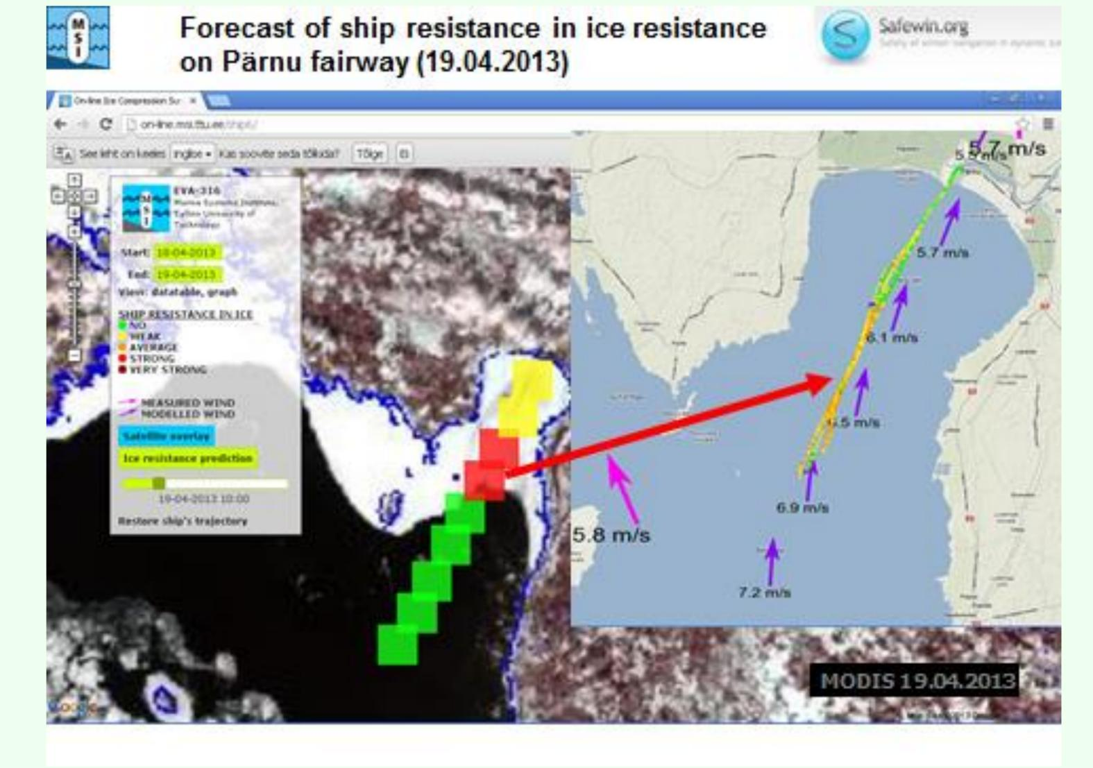
Screenshot of web based user interface for forecast of ice compression hazard (ship resistance in ice) implemented in fairway into Pärnu Harbour, Gulf of Riga. MODIS satellite data were used to give ice situation as background and different colors show grading of ship resistance forecast, hourly for 48h ahead. The pasted figure shows the *in situ* measurements of ice resistance index (one option of web based user interface).
