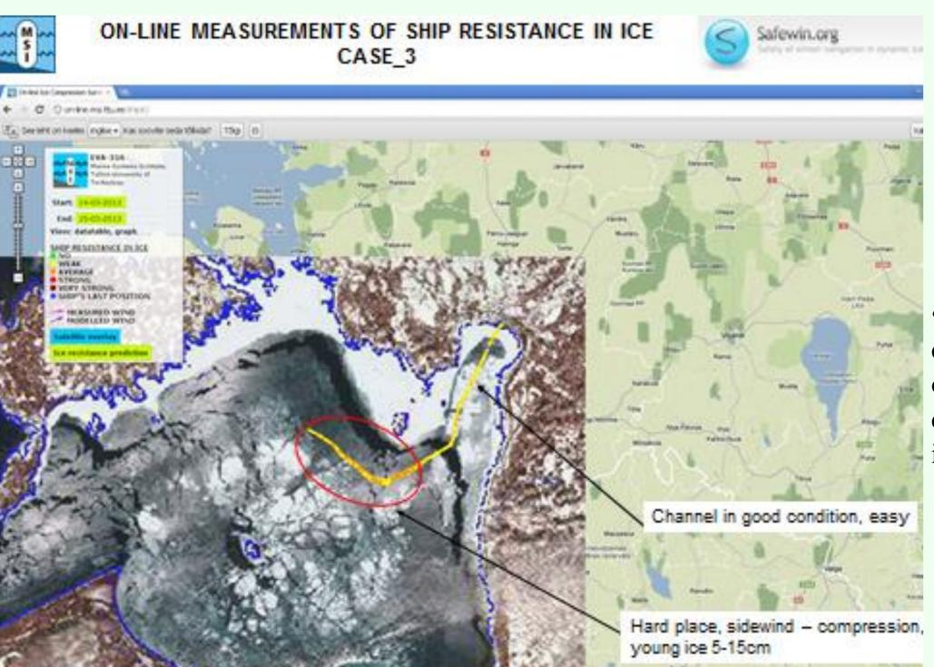
•The angle between the wind direction and ship course is one of the important factors determing the ship resistance in ice channel
